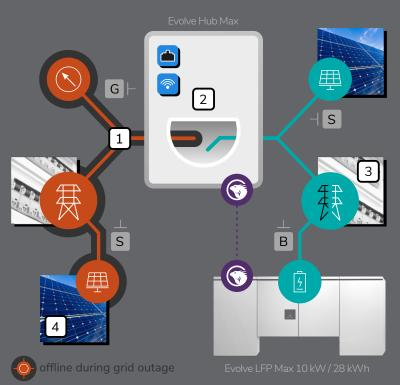
PV inverters rated up to 15.4 kW AC with power limiting<sup>-2</sup> to 10 kW AC during backup operation may be connected to the Evolve Hub Max.
