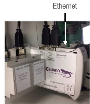
Figure 11: Droplet Ethernet connection.
